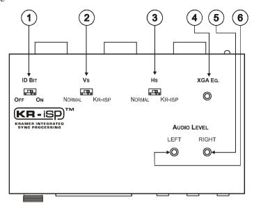
Figure 4: VP-200NAK 1:2 XGA / Audio DA (Underside)
